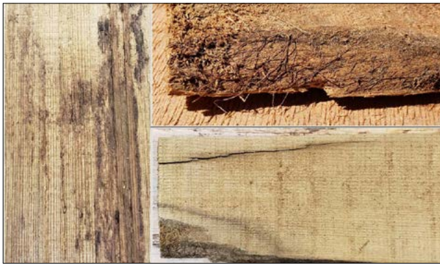
Figure 4a. Dark-pigmented fungi color the surface of these cedar shingles.
