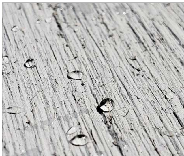
Figure 7. Water beads on the surface of wood treated with a water-repellent wood protection system.
