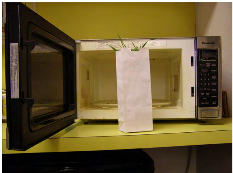
Figure 2. A forage sample in a paper bag ready to be dried in a microwave oven.
