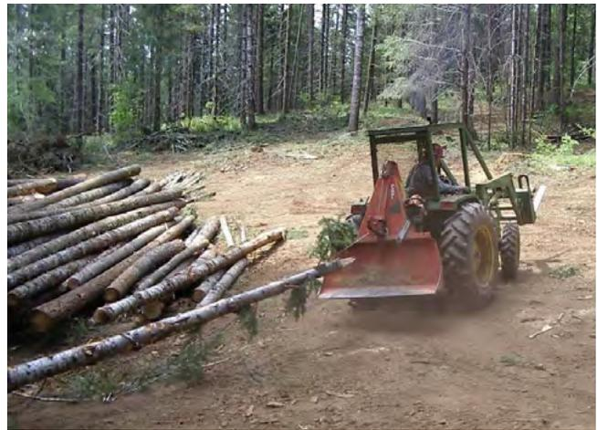
Many small-scale operations use machinery not typically associated with logging activities. Farm tractors, for example, can be equipped with various accessories employed in logging. In this photo, a Farmi winch is being used to skid logs.
