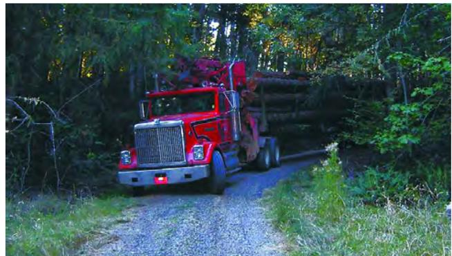
Clearance requirements for personal vehicles are much different than those for logging trucks and logging equipment, especially in terms of turning radius and steepness.
