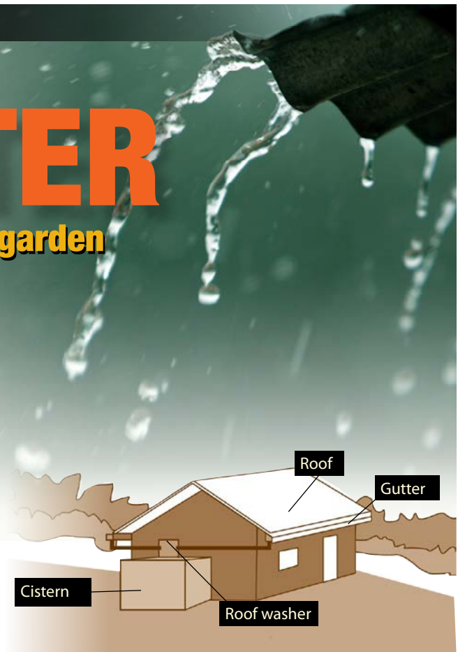
Figure 1. Above-ground rainwater collection and storage system.
