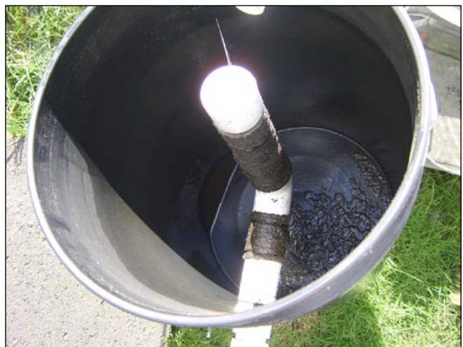
Figure 9b. Rainwater contains many roof contaminants that easily get trapped in this homemade filter made from air and dust vent filter material.
