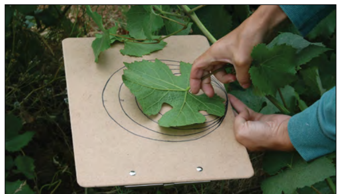
Figure 5. When measuring the size of each leaf, center the whole leaf on the respective circle to determine size as shown. The circle that best fits the leaf size should be recorded on the data sheet. For example, the leaf shown above should be recorded as a category 2 leaf. (Photo: Patricia A. Skinkis, © Oregon State University)
