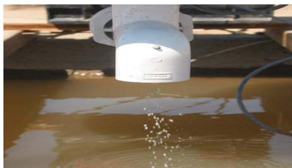
*Figure 7. Applying PAM with a metered dispenser.*
