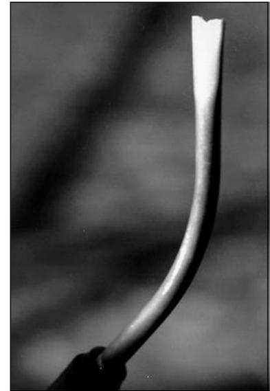
*Figure 4.—A new tip can be constructed using a  $\frac{3}{8}$ -inch pipe nipple and coupler. Note the end of the nipple has been smashed flat, creating an opening of about  $\frac{3}{8}$  inch for the flame. This allows the gas to burn cool with no aeration. Remove the end of the weed burner and attach the new tip to the end of the torch.*
