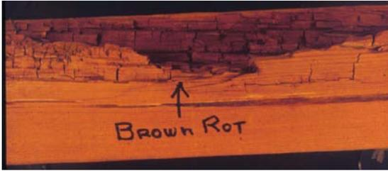
Figure 4. The final stage of wood decay by the brown rots can be identified by the dark brown color of the wood, excessive wood shrinkage, cross-grain cracking, and the ease with which the dry wood substance can be crushed to powder.
