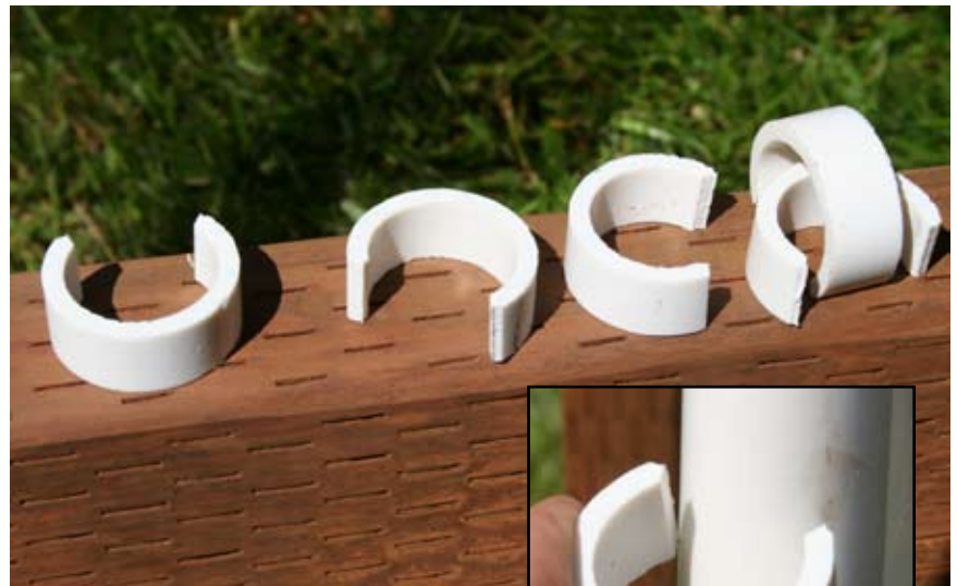
Figure 7. PVC clips for attaching polyethylene plastic sheeting to the ends of the cloche.
