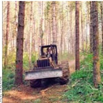
Figure 3.—Harvesting with a rubber-tire skidder.
