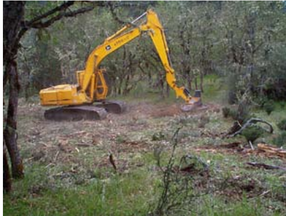
Figure 1. Slashbuster equipped with rotating head. Photo: Ed Reilly, Bureau of Land Management.
