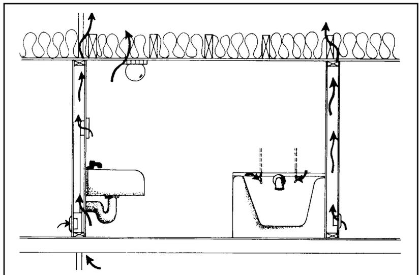
Figure 3. — Attic bypasses from the bathroom.
