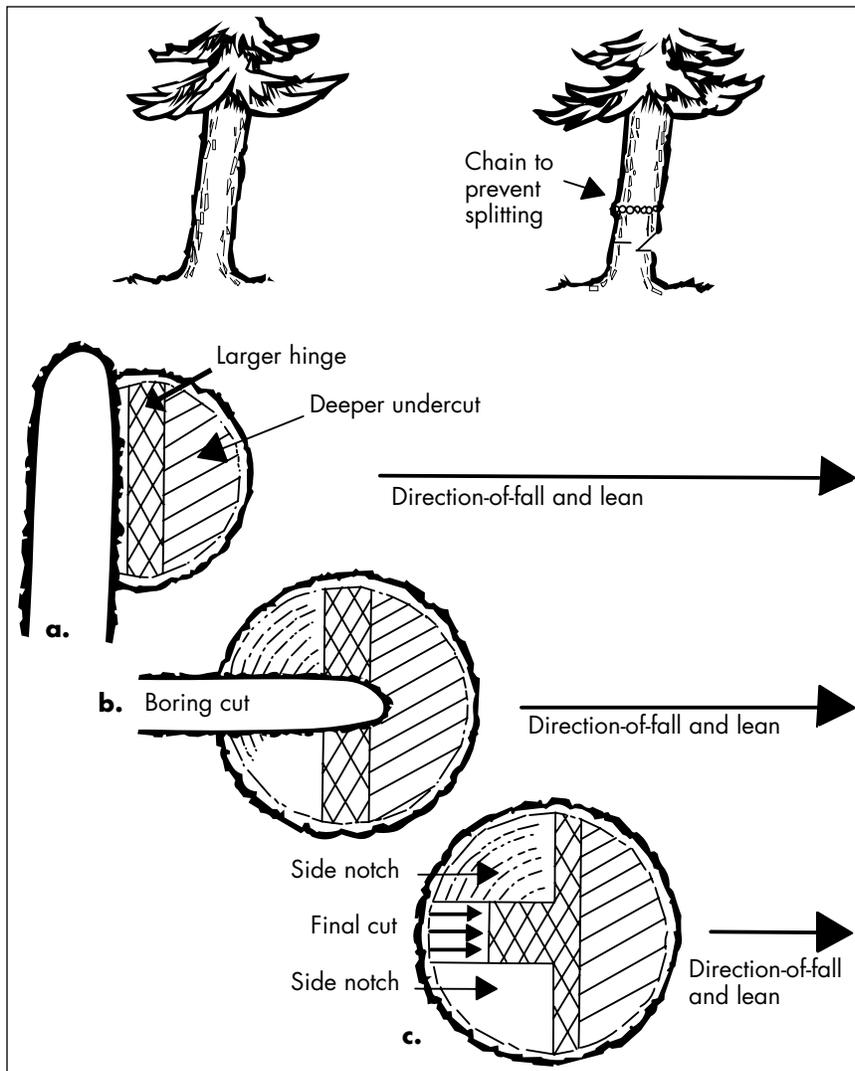
Figures 17a-c.—Three options for back cuts in order to fell a leaning tree in the direction of the lean.
