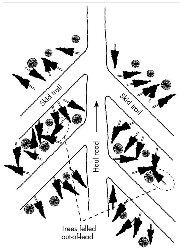
Figure 1.—A planned felling pattern (not to scale).
