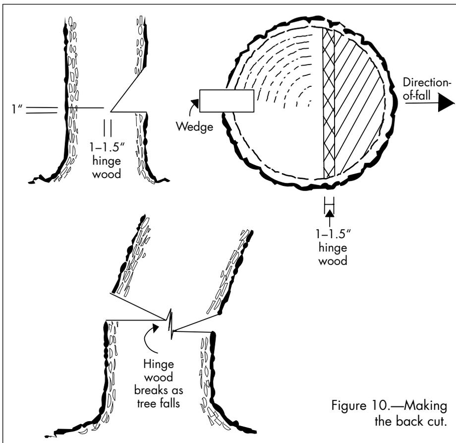
Figure 10.—Making the back cut.
