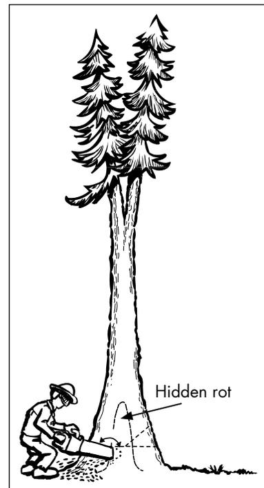
Figure 3.—Boring the stump to detect rot inside.
